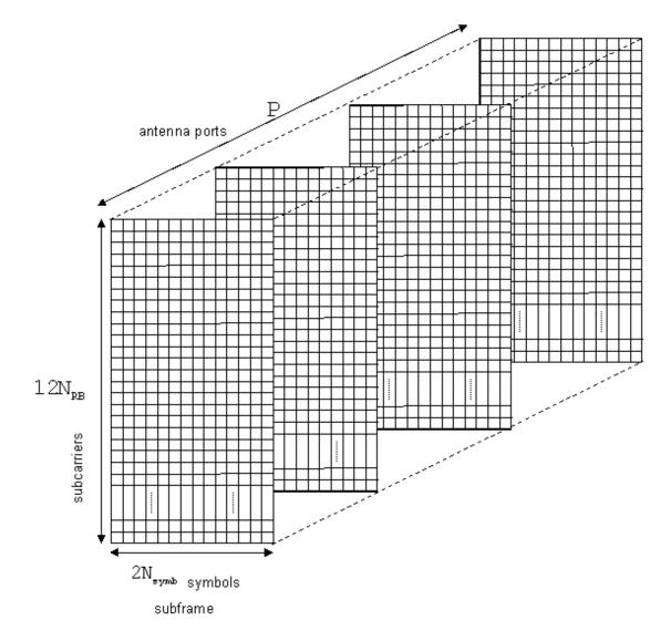
The rows of this array represent the subcarrier. The columns map the OFDM or SC-FDMA symbols in the downlink and uplink, respectively. The third dimension or plane represents the antenna ports. In the LTE System Toolbox, the resource grid spans a subframe in the time-domain, instead of a slot. Hence, the documentation uses the term
